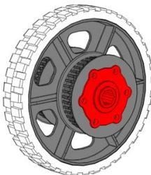
**Step 6:** Add six 10-12 x 1.5" (am-1654) thread forming screws to attach the pulley and hub to the wheel.
