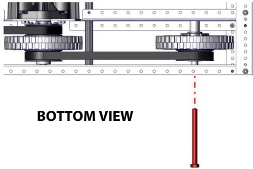
**Step 24:** For the belt runs that are closest to the Inside Plate, the Short Axle Spacer (am-1306) will be closest to the Inside Plate. The Long Axle Spacer (am-1307) will be closest to the Outside Plate.
