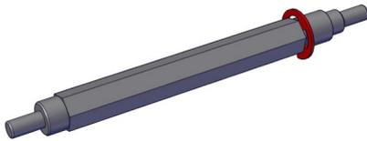
**Step 6:** Insert the end closest to the E Clip of the TB Hex Output Shaft into the other R6ZZ bearing.
