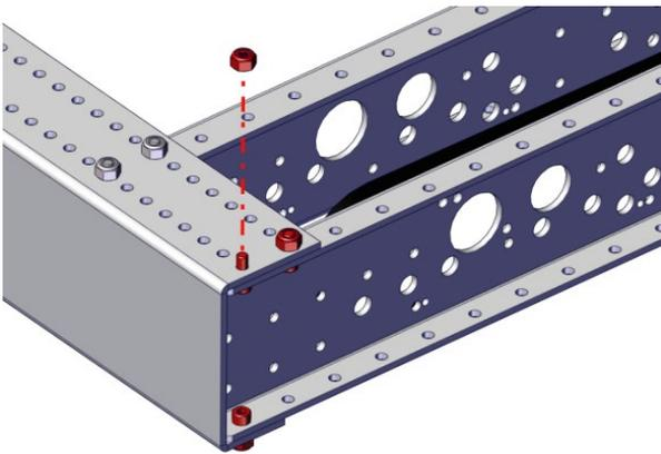
**Step 17:** Attach four 3.375" Churro Standoffs (am-2569) (see below for recommended locations) with 1/4-20 x 0.75" Thread Forming Screws (am-1310) onto each Inside Plate. A 1/2" wrench can be used to hold the churro while tightening. Make sure to loop belts over the churro to ensure the belts have a straight path from axle to axle.
