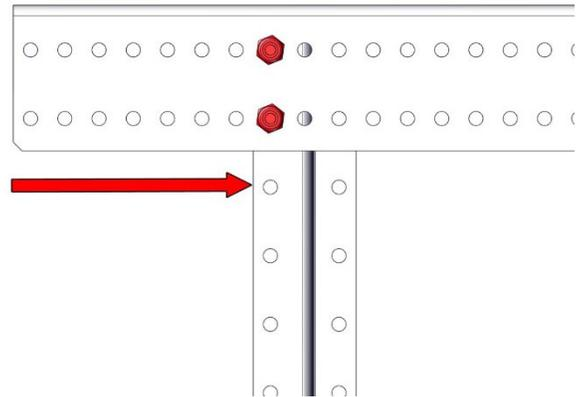
**NOTE:** The top flange of the Inside Plate should point toward the short side of the End Plate
