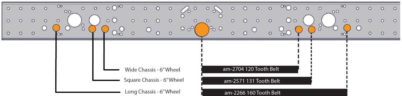
**NOTE:** Axle bolts must be installed from the outside of the chassis. If they are inserted into the Inside Plate first, the standard bumper hardware will not fit.
