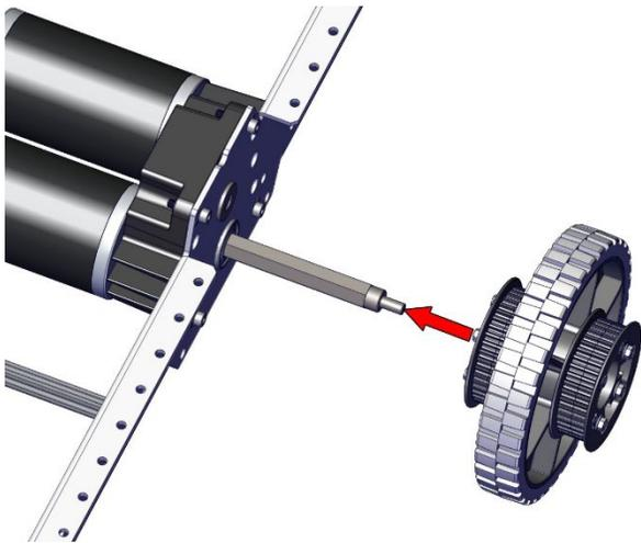
**Step 10:** Line up the CIM motors with the mounting holes in each ToughBox Mini S. Secure each motor with gears installed to the ToughBox Mini S housing using two 10-32 x 0.625" SHCS w/ Nylon Patch (am-1120).
