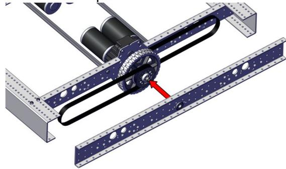
**Step 16:** Secure the Outside Plates to each End Plate using six 10-32 x 0.500 socket head screws (am-1002) and six 10-32 Nylock nuts (am-1042).
