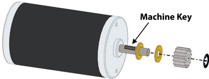
**NOTE:** Each drive gearbox can accept up to 2 motors. Repeat this step for each motor.
