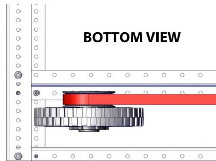
**Step 25:** Slide a  $\frac{3}{8}$ " axle bolt (am-1297) through the spacers and wheel assembly, with the head of the bolt on the outside of the chassis.
