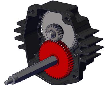
**Step 9:** Apply Red Tacky Grease (am-2768) to all of the gear teeth.
