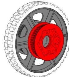
**Step 5:** Insert one 1/2" Hex Hub (am-2568) into the pulley on one side of the wheel.
