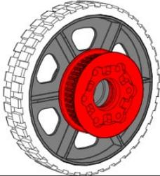
**Step 2:** Using six 10-12 x 1.5" (am-1654) thread forming screws, attach the pulley halves to the wheel.
