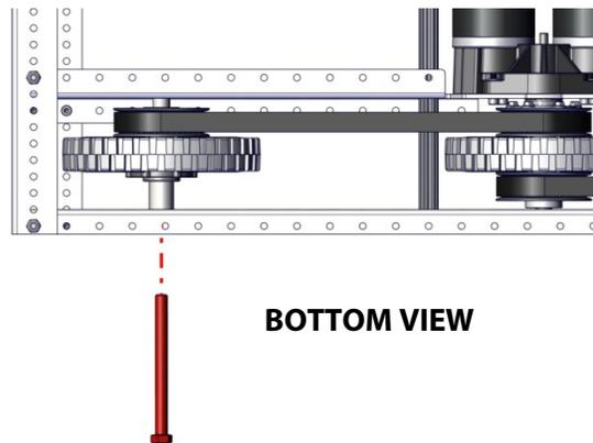
**Step 27:** Repeat steps 19 through 26 to install wheels on other side of chassis.
