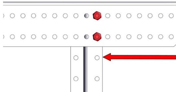
**NOTE:** The top flange of the Inside Plate should point toward the short side of the End Plate
