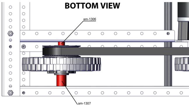
**Step 26:** Install one  $\frac{3}{8}$ -16 Nylock Nut (am-1054) on each Axle Bolt. Tighten the bolt and nut until the spacers just begin to touch Inside and Outside Plates. The wheels should still easily turn, and the axle bolts should be able to spin with a light turn of a wrench.
