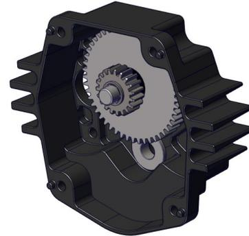
**Step 5:** Tap the 1/2" E-Clip (am-0206) into the groove on the TB Hex Output Shaft.
