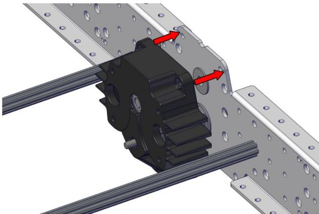
**Step 8:** Attach one ToughBox Mini S to each Inside Plate with four 10-32 x 0.75" SHCS (am-1047) and four 10-32 Nylock nuts (am-1042). The nuts will fit into the hex pockets on the ToughBox Mini S housing and will hold the nut while tightening.
