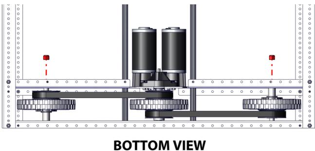
**Step 23:** Add another Outer Wheel Assembly to the other end of the chassis. Loop the belt onto the pulley and insert the assembly between the Inside and Outside Plates. This assembly should have its pulley facing opposite of the first assembly.
