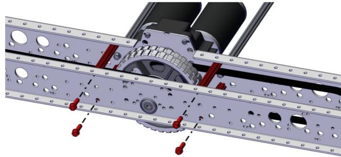
**Step 19:** There are different axle bolt locations for each chassis configuration. Locate the hole to match the chosen belt and frame size.
