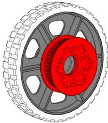
**NOTE:** Tighten the screws in a star pattern to ensure the pulley aligns evenly on the wheel.
