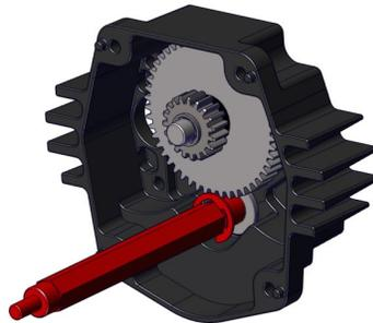
**Step 8:** Place the 45 Tooth Gear (am-4712) on TB Hex Output Shaft.
